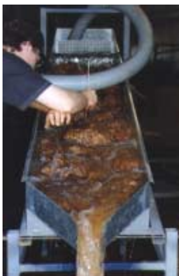
Laboratory Erodibility Testing of ferricrete erodibility in flumes, showing visible armouring of the ferricrete.
