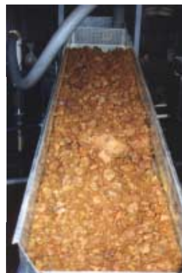
Laboratory Erodibility Testing of ferricrete erodibility in flumes, showing visible armouring of the ferricrete.
