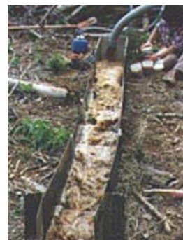
Testing effectiveness of Hoop Pine litter — sediment samples taken at the flume inlet and outlet.
